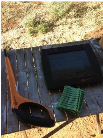
*The reader, in this case a Gallagher HR4 stick reader is used to transfer information from the RFID tag to an indicator.*
